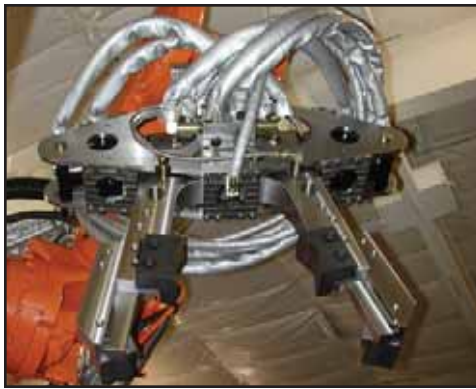
Close-up of end-of-arm tooling on a new forging robot.
