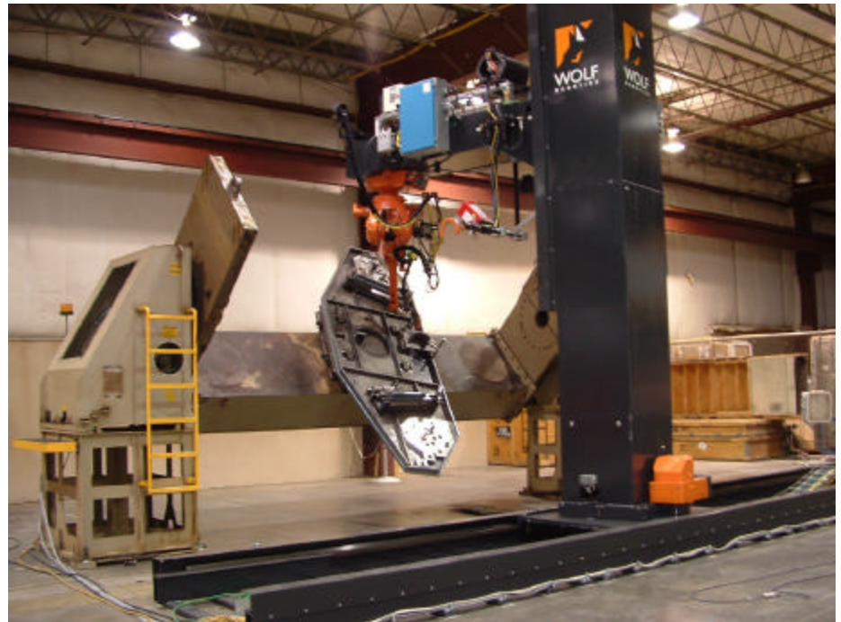
Existing Heavy Duty 2 Axis Positioner and new Robot Rotating Tower & Travel Track combine old components with new technology at a reduced cost.
