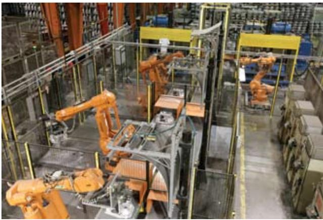
*The robots work in conjunction to maximize efficiency, accuracy, safety and consistency in this finishing cell that is automated with two twin presses, six robots, a large conveyor and shotblast.*
