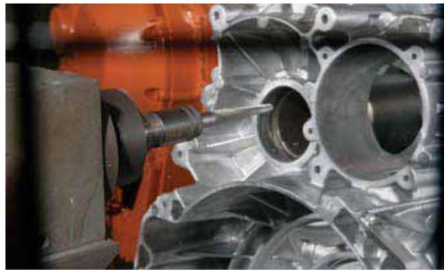
*Due to the precise and efficient nature of robotic finishing, Ryobi Die Casting has reduced hand filing by 85 to 90 percent in recent years.*
