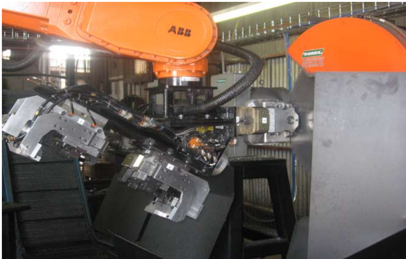
The first gripper is used to saw the runners and risers and separate the casting. The second gripper presents each casting individually to the deburring spindle for removal of heavy flash.
